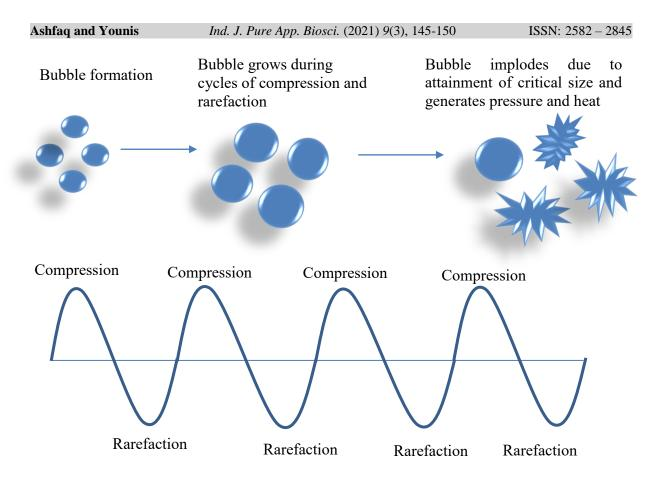
Figure 1: Generation of cavitation bubbles due to the propagation of sound waves via series of compression and expansion
